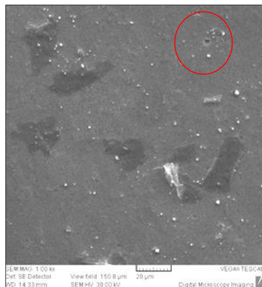
Figure 16. Pores present on Zy-4 (Y2-77).
