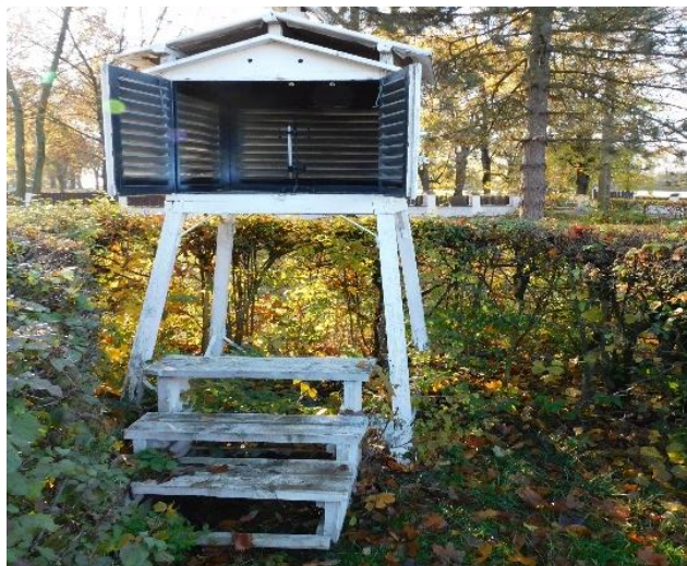
Figure 4. Classic air temperature monitoring station.
