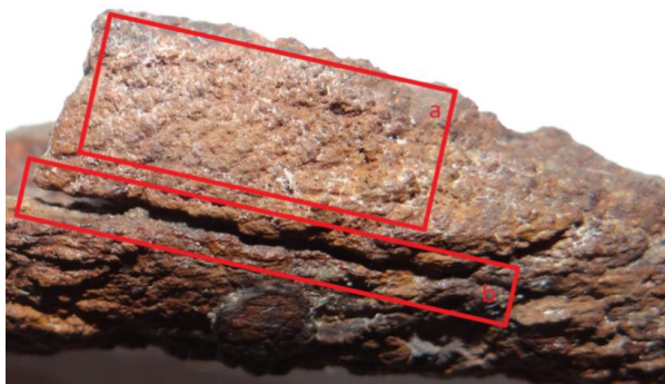
Figure 2. Macroscopic image: a) Textile pattern; b) the joining area of the metal sheet.
