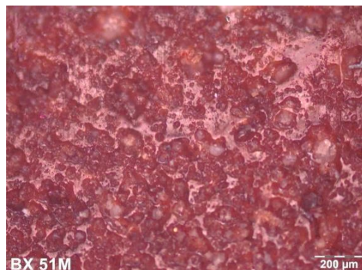
Figure 25 Surface microstructure of C6 after vibration testing: 4h, 330Hz, 15.7 m/s 2 , M 100X
