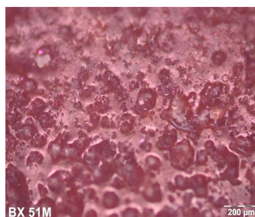
Figure 19. Surface microstructure of C3 after vibration testing: 4h, 330Hz, 15.7 m/s 2 M 100X
