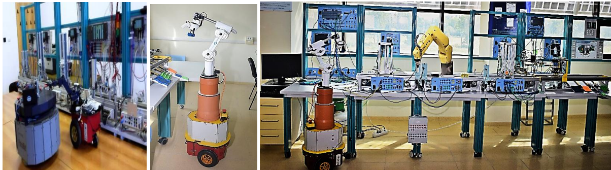
Figure 1. Assembly/Disassembly stations from SMART&ASTI A/DML served by MRs
