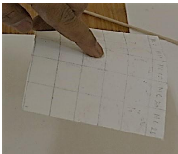
Figure 1. Canvas got pulled along the gel residue due to high adhesion at 15 and 20% concentration of MC gels.
