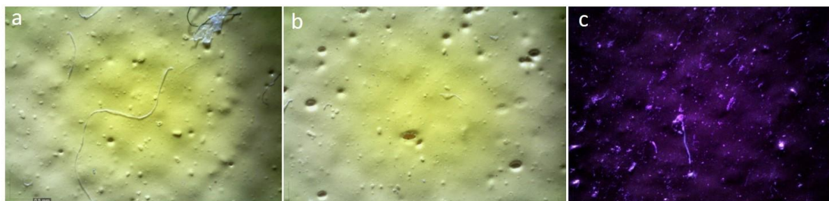
Figure 4. a) Image showing the presence of methylcellulose residue; b) image showing some pitting occurred with a digital microscope in sample cleaned with MC 10%; c) ultraviolet image showing some cotton fibres adhered on the sample cleaned with MC 25%.
