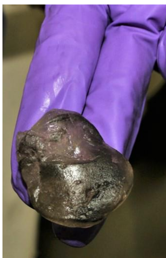
Figure 3. MC at 25% concentration behaving as a molecular trap and lifting the dirt in its matrix.
