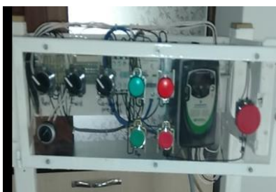
Figure 19. Internal components of the drive stand
