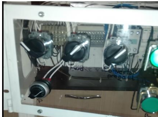
Figure 24. Starting the asynchronous motor in a certain direction, with a certain speed and the P potentiometer that simulates the pressure transducer
