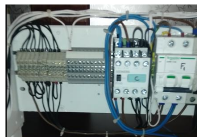
Figure 18. The front panel of the drive stand contains the electrical control and signaling components and is mobile
