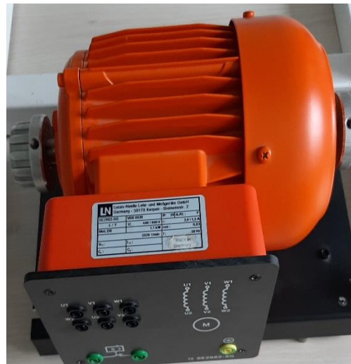
Figure 4. Three-phase asynchronous motor with short-circuited rotor used to design and build the experimental stand
