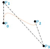
Figure 2. Rational Cubic Bezier Curve.
