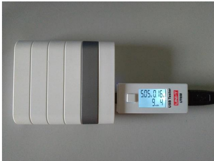
Figure. 13. The experimental MCT system connected to a 10200mAh power bank, through an USB digital power meter – reading a constant voltage of 5.05V_{DC} and a 0.16A current draw, while conducting the ECG measurements.
