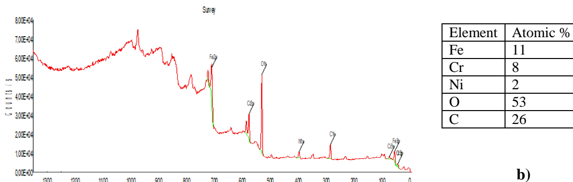
Figure 6. The survey spectra of 304L-N and 304C before Argon ion etching: a) 304L-N sample; b) 304-C sample.
