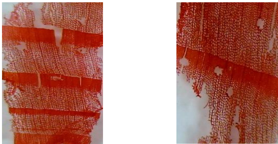
Figure 15. Thin section micrograph of wood from the investigated ceiling illustrated that it belong to the Pinus wood, 40X.
