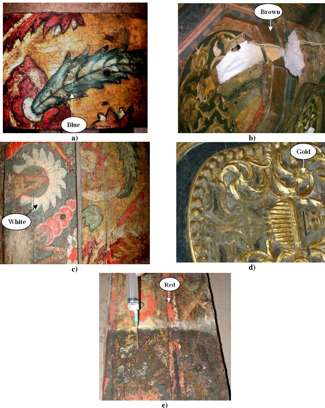
Figure 4. Pigment samples from the wooden ceiling of Abdel Rahman Katkhoda
