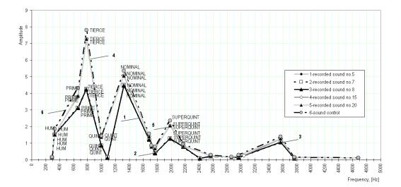
Fig. 1. Frequency dependence of the amplitude of the main partials versus sound control sample (no. 6)
