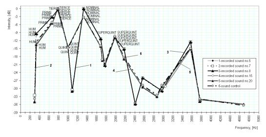
Fig. 2. The influence of frequency variation on the intensity of the main partials recorded versus sound control sample (no. 6)
