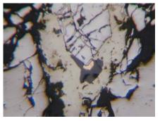
d) Native gold at the boundary between quartz and arsenopyrite, in chalcopyrite. Valea lui Stan ores. N II, 190x magnification, oil imersion.
