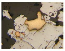
a) Gold inclusions in arsenopyrite. Valea lui Stan ores. N II, 120x magnification.
