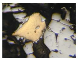
b) Gold with arsenopyrite inclusions. Valea lui Stan ores. N II, 120x magnification.
