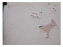
e) Native gold and pyrrhotite in arsenopyrite. Costești ores. N II, 190x magnification, oil imersion.
