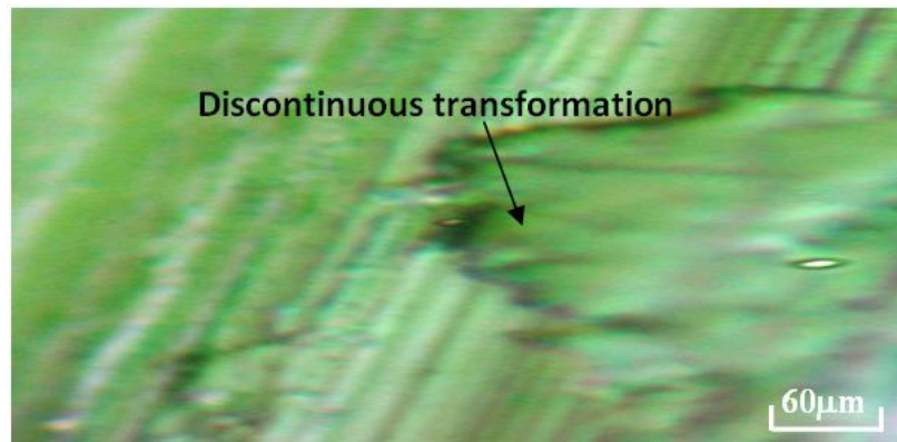
Figure 6. Quenching structure evolution of Pb 1, 5% Sb 0, 8% Al as-cast alloy at 20°C. Visualization of discontinuous transformation after 22 minutes.
